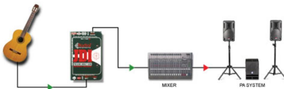
In its simplest form, the instrument connects to a DI box and the XLR output is connected to the PA system. The primary advantage of using a DI versus connecting directly is noise. Balanced lines are much less susceptible to picking up noise from lighting systems, dimmers, motors and so on. As a rule, high impedance cables should not exceed 8 meters (25 feet).
